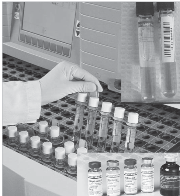
Figure 1. BACTEC MGIT (mycobacterial growth indicator tube) system – MGIT machine; upper right inset, MGIT tubes; lower right inset, antibiotics solutions for performing susceptibility testing in MGIT.
